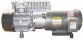
Model TV 25B Displacement 21 CFM Ultimate Pressure .5 Torr
